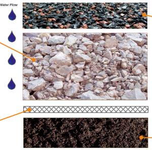
A FlexiSet aggregate size of 6mm requires a standard depth of 35mm
