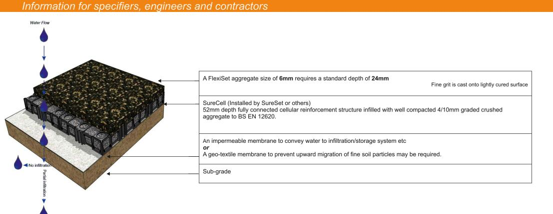
Full infiltration - water returns to sub-grade Partial infiltration - impermeable membrane used to convey water to storage tank for either storage or controlled release
