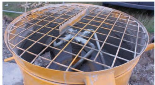
The "Continuous Mixer" is a "forced action" mixer which comprises a hopper and connected screw-feed blending tube into which water is continually fed and which delivers ready-to-use mortar on demand.
